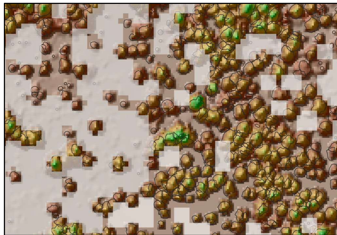
Figure 1. Example of gap delineation overlaying a CHM and segmented trees in 1.8-acres of unit 28. Tree height is shown with the brown-to-green color ramp while gaps are in greyscale. Gaps can be large and convoluted (left) when areas are connected narrow regions.
