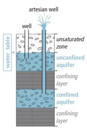
Aquifers can be both confined and unconfined. Unconfined aquifers are usually shallow. In an unconfined aquifer, the water table is the top of the aquifer and is only subject to atmospheric pressure (just like surface water). Confined aquifers are usually much deeper and are constrained by dense rock from above and below that limits groundwater flow into or out of the aquifer. This can cause the aquifer to be pressurized beyond atmospheric pressure.
