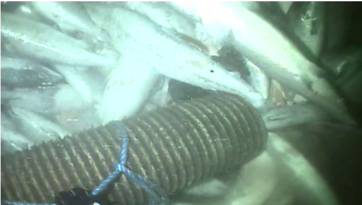
Figure 31. Screenshot from Dive 5 on August 26. This shows optimal conditions for obtaining an accurate count of fish extracted: camera is pointed directly at opening of suction pipe, fish are whole, and there is little debris (decomposing fish) in the water.
