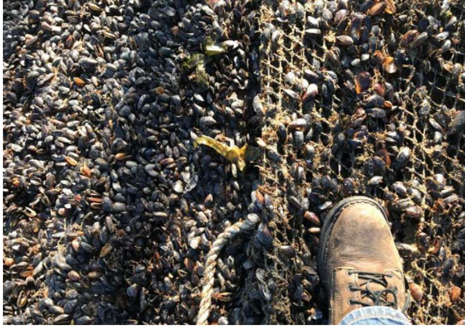
Figure 14. Stock net retrieved following August failure, photographed on September 1 in Anacortes. Note heavy fouling by mussels.
