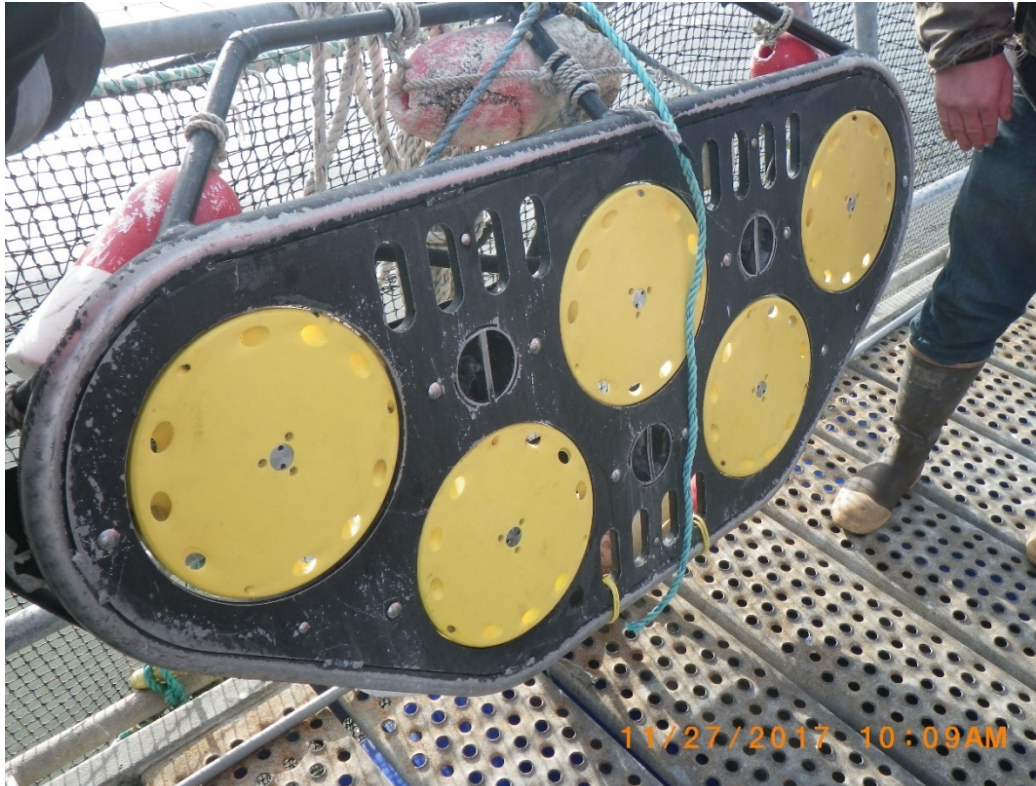
Figure 11. MPI net cleaning machine at Hope Island farm on November 27, 2017. Pressurized water rotates the five yellow heads.
