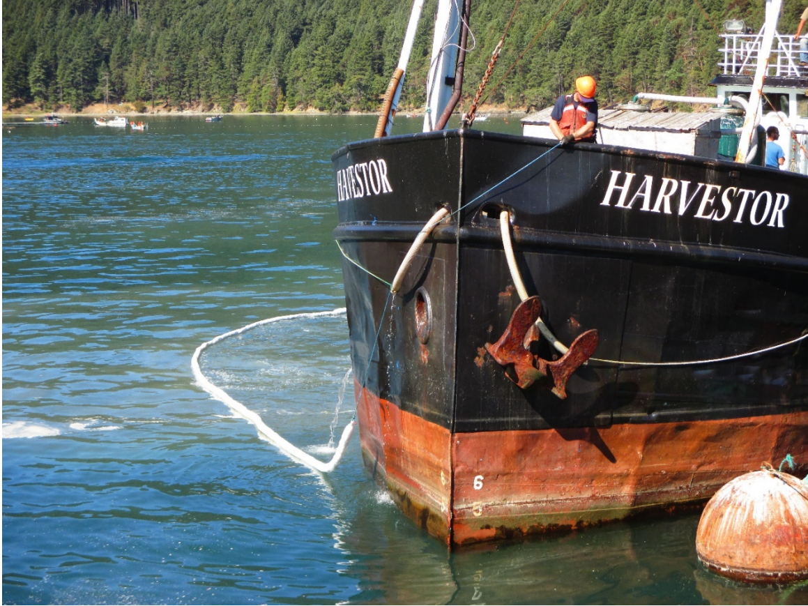
Figure 24. F/V HARVESTOR on August 26, 10:31 a.m. First day of fish extraction onto vessel. The forward draft is about 4 feet.
