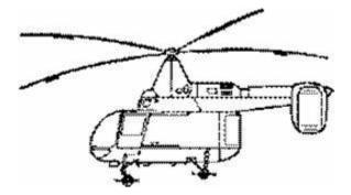
The Kaman could be designed extremely compact because of it's bi-rotor system. Between 1958 and 1965 some 365 were built.
