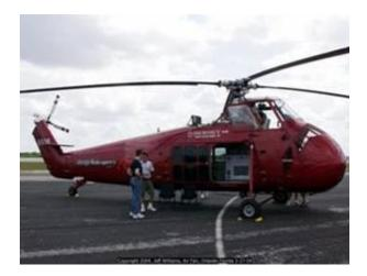
The Sikorsky S58 (H34) Choctaw was the only one used by DNR in 1971 and offered extended capability for providing larger crews and greater water capacity. This helicopter carried a 450 gallon bucket and had a 1500 horsepower engine.
