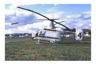
The Kaman Husky replaced the Bell 47s in DNR fire use in 1974. The Kamans continued to use the Sims 450 gallon bucket, normally carrying 300 gallons (plugs removed). At various times six Kamans were stationed across Washington State. Three in Western Washington (Castle Rock, Enumclaw, and Sedro Woolley), and three in Eastern Washington (Ellensburg, Omak, and Deer Park). The ships generally operated with a crew of 2-4 firefighters. The Huskies started
