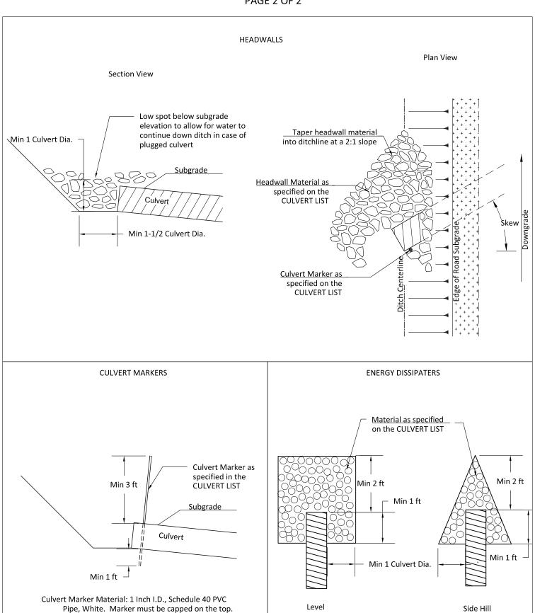
Min Energy Dissipater Depth: 1 Culvert Dia.
