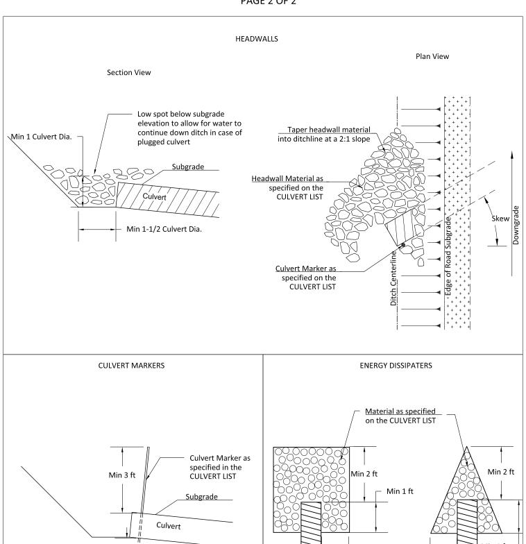
Culvert Marker Material: 1 Inch I.D., Schedule 40 PVC Pipe, White. Marker must be capped on the top. Culvert Marker Placement: Place on uphill side of culvert, between corrugations if possible.
