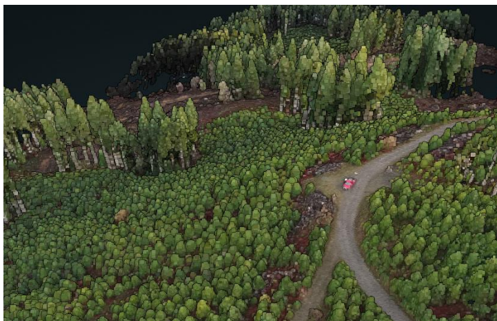
Figure 18: A Photo Point Cloud Derived from Aerial Imagery Taken by an Unmanned Aircraft System. Photo courtesy of Jacob Beard.
