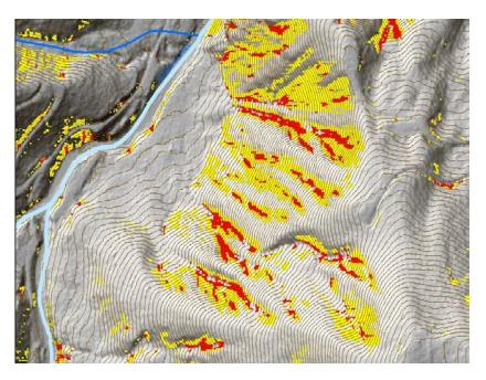
Example output from the LiDAR-based SLIPS tool
