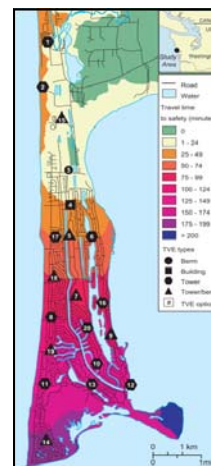
Study area map of Ocean Shores, Washington, including modeled pedestrian travel times to safety, vertical-evacuation sites proposed during Project Safe Haven meetings, and regional map.
