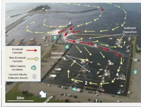
Figure 2: Tsunami flow-regime map for Crescent City Harbor. Current directions and velocities, and areas of sediment erosion and deposition are based on observations of the various (30) ground-level and aerial video, pre- and post-tsunami bathymetry, and sediment analyses (modified from Wilson et al, 2012b).
