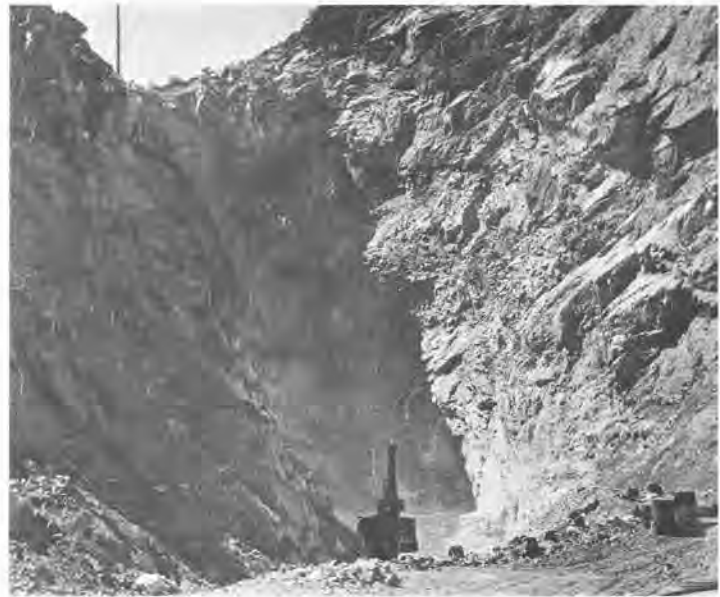
FIGURE 11.— Shelf and pit quarry, Marble No. 2 deposit, Grotto, King County. Steeply dipping narrow limestone bodies pose many problems in quarrying.
