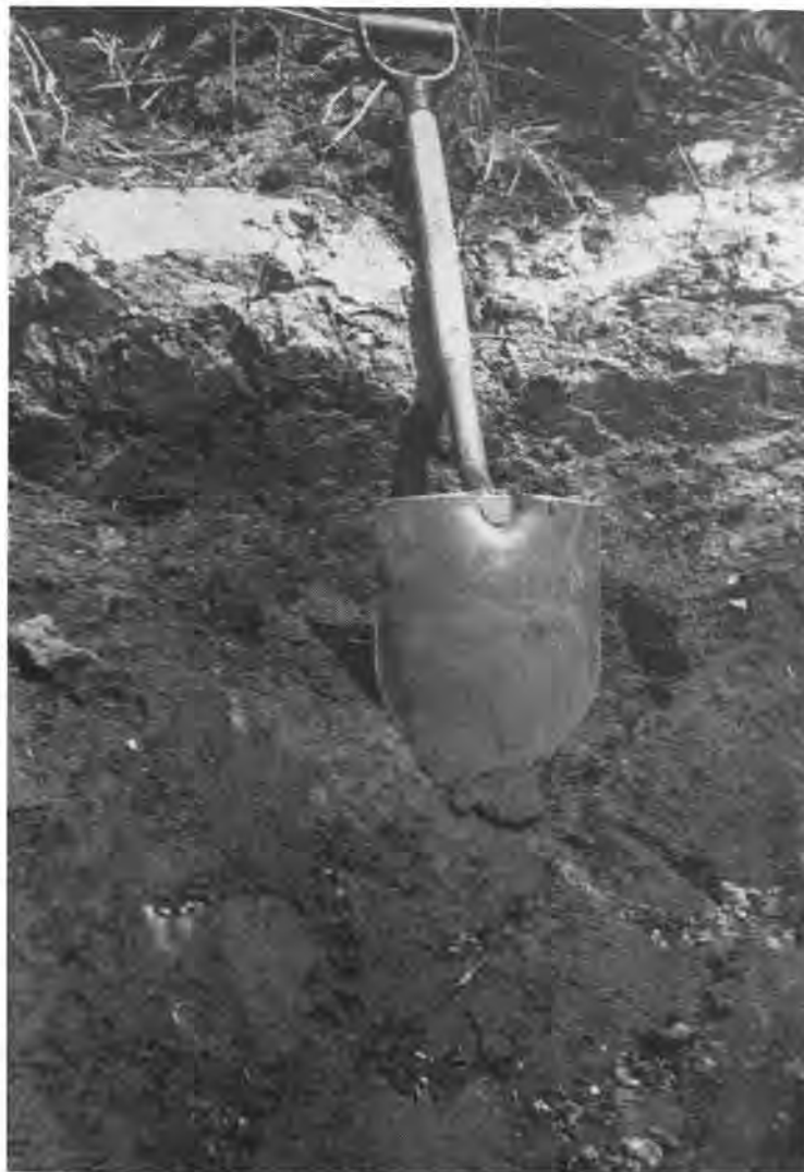
FIGURE 71.—Part of bank of excavation in Seola peat deposit (28th Avenue S.W. and 104th Street S.W., Seattle). Layer of white diatomite, approximately 3 inches thick, 18 inches below surface. Layer of brown pumicite (dark color) below diatomite. Top and bottom of bank not shown.
