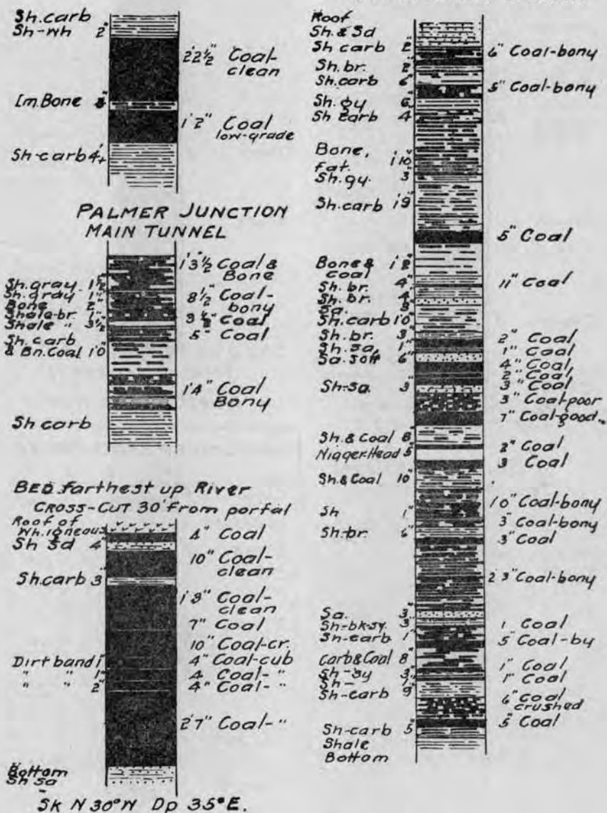
FIG. 38. Cross-sections of Coal Beds near Palmer Junction.
