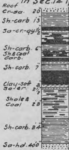
FIG. 39. Cross-sections of Coal Beds near Palmer Junction.
