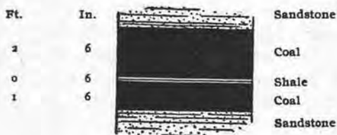
Fig. 11. Cross-section of vein, Raging River Field, Secs. 25 and 26, T. 23 N. R. 7 E.
