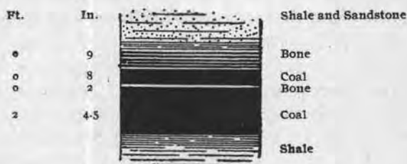
Fig. 20. Cross-section of No. 1 vein, Sunset Mine.
