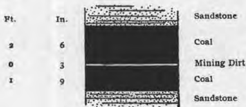
Fig. 22. Cross-section of No. 4 vein, Burnett Mine.
