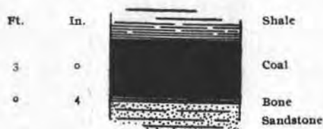
Fig. 13. Cross-section of Gem vein, Franklin Mine.
