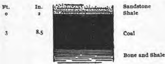
Fig. 23. Cross-section of No. 5 vein, Burnett Mine.
