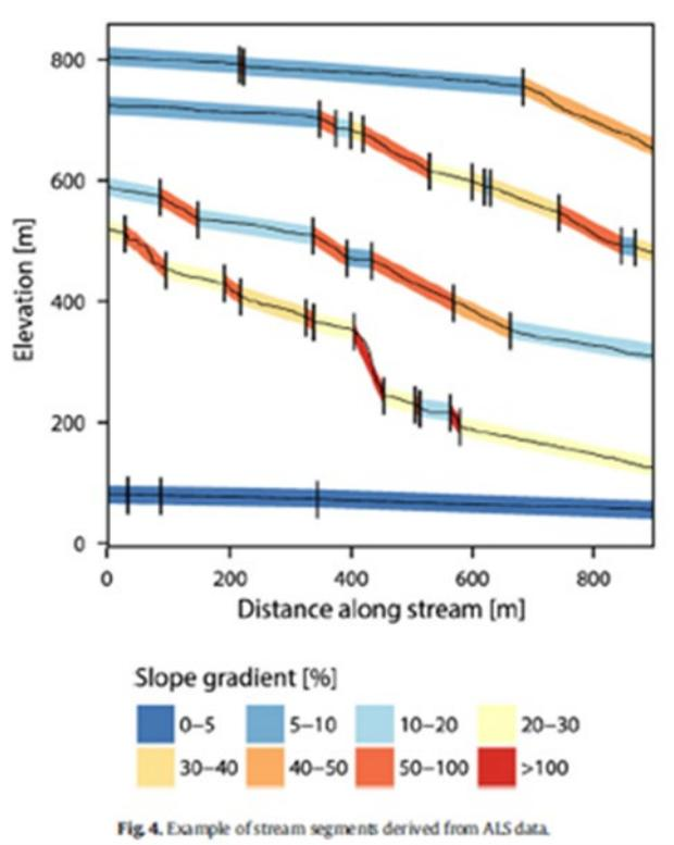
**Figure 1.** An example of channel segmentation of varying length having homogeneous channel gradients (Tompalski et al. 2017). Appropriate gradient breaks will be defined during consultation with project collaborators.
