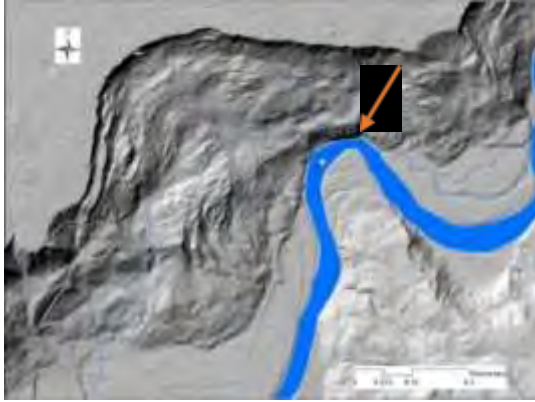
Figure 26. LiDAR image showing channel incision within a large deep-seated slump feature in the Tolt River valley, King County.
