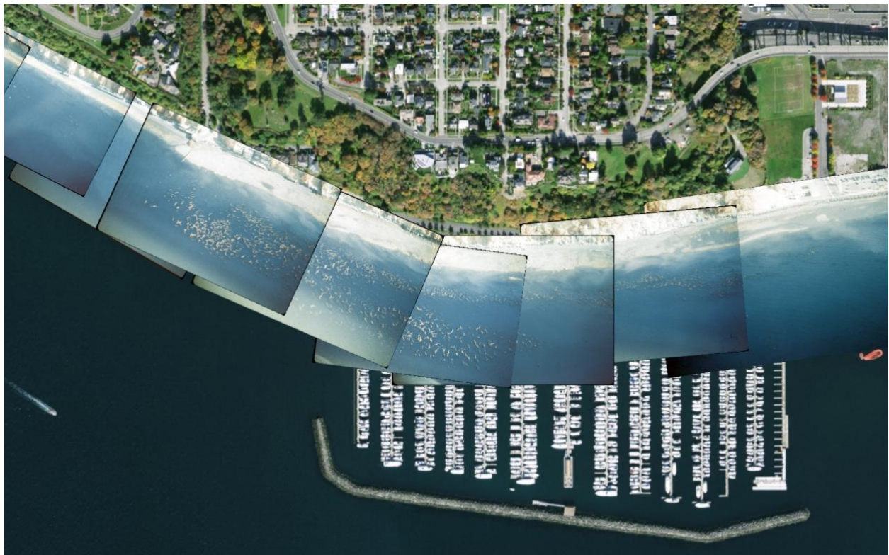
Figure 7. View of 1984 images placed along shoreline at Magnolia. Images have been moved, rotated, and scaled to maximize alignment of notable shoreline features with reference imagery and with neighboring images, but have not been transformed or rectified relative to the ground. Underlying imagery is 2019 NAIP Natural Color Imagery Basemap (Esri, USDA Farm Service Agency).
