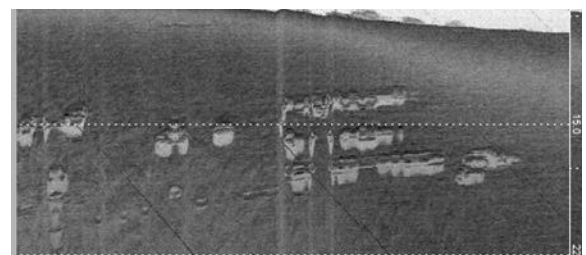
Figure 2. Side-scan data collected with a Triton Starfish 990F side scan sonar. Rows of tires can be seen in the area.
