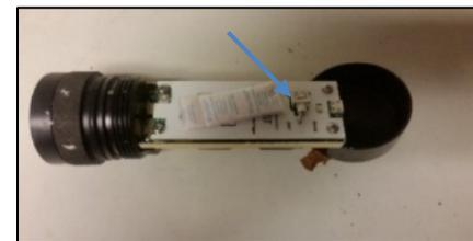
Figure 12: Chlorophyll sensor, blue arrow point to on-off switch
