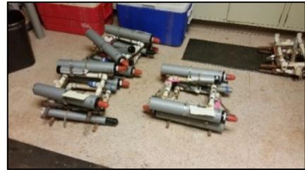
Figure 11: DO sensors, arrow point to hose clamp and logging lever
