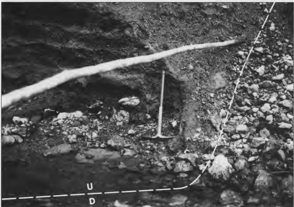
Figure 5. (See Figure 3 for location.) Truncated colluvium exposed in the south bank of an unnamed tributary to the Canyon River. Note the apparent drag folds in clay layers to the right and left of the 66-cm pick handle. The deformed clay layers contain abundant charcoal and are separated by coarser colluvium. The approximate fault trace is shown by the dashed line. At this locality, the fault trace is easily recognized in the stream bed because the upthrown block is scoured to sheared basaltic bedrock, but the younger alluvium has deposited in the present channel adjacent to the scarp. Shears within the basalt project from left to right directly toward the deformed clay beds.
