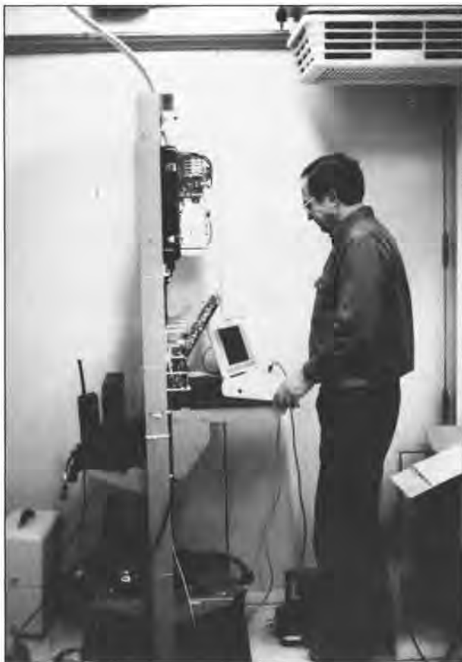
Figure 1. Leroy Foote of the U.S. Geological Survey tests the controller station for the strong-motion accelerometers in the Natural Resources Building.
