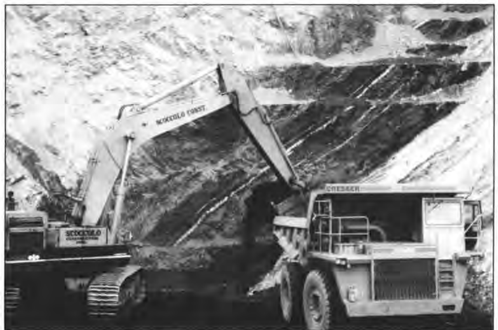
Figure 2. John Henry No. 1 mine, Pit No. 1, January 1993. Coal from the Franklin Nos. 7, 8, and 9 coal seams where they have merged on the southeast limb of an anticlinal fold is being mined with a mass excavator. The thin, light-colored bands within these bituminous coal measures are volcanic ash beds. Coal is hauled by truck to a beneficiation plant located \frac{1}{3} mile from the pit. For other views of the anticline as it was exposed in the pit, see p. 31, vol. 17, no. 1 (photo taken August 1988); p. 27, vol. 19, no. 1 (November 1990); and p. 26, vol. 20, no. 1 (January 1992).
