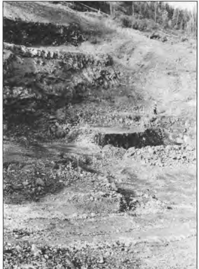
Figure 9. Stripping overburden and mining began in the fall of 1992 at the Key West deposit owned by Echo Bay Minerals. Ore, exposed in the center of the photo, consists of magnetite with subordinate pyrite, pyrrhotite, and chalcopyrite. Mining at this and the nearby Key East deposit is scheduled to be completed in early fall of 1993. Ore reserves at these deposits are almost 900,000 tons and contain more than 100,000 ounces of gold.
