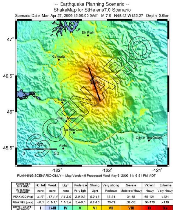
Figure 1. ShakeMap for a M7.0 earthquake on the St. Helens seismic zone. The heavy black line is the modeled fault for this scenario.
