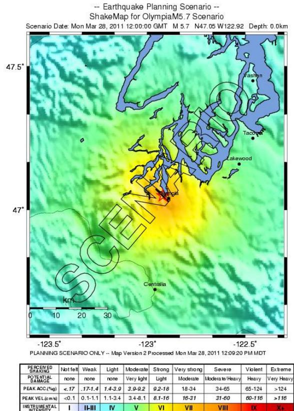
Figure 1. ShakeMap for a M5.7 earthquake on the Olympia fault.
