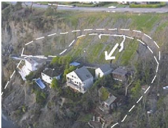
Figure 8: Deep-seated slide in Seattle, WA (above) (WDGER photos). Bowing trees that indicate deep-seated slide movement south of Holly (right).
