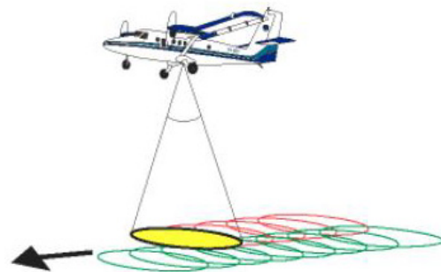
Figure 13: LIDAR data acquisition with rangefinder installed in fix-winged aircraft (modified from PSLC, 2000).
