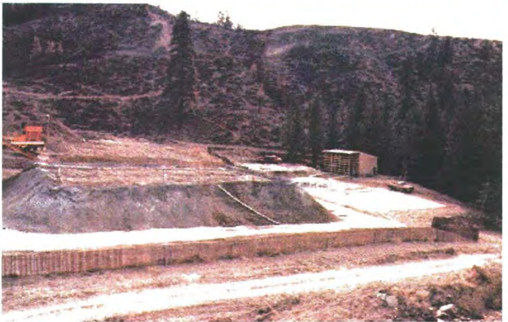
Figure 15c. Ore stacked 16 feet high on the only pad that was actually used at the Minnie mine. Ore was crushed and agglomerated with cement prior to stacking. Sprinklers delivered cyanide solutions. Spent ore was washed with water and also neutralized using alkaline chlorination. During reclamation, stripping neutralized layers off the pad assisted neutralization by exposing lower material to air, light, and treatment solutions. (Photo by Rod Lentz, U.S. Forest Service, Okanogan National Forest.)
