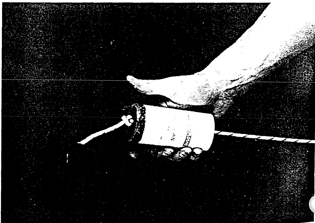
Figure 3-5. Detonating cord with the Atlas G booster. (Reprinted from Atlas Powder Company, 1987, Explosives and Rock Blasting, figure 8.19.)
