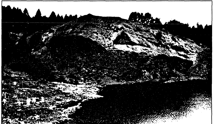
Figure 5. Shot holes drilled to progressively shallower depths provide a blast pattern that will reduce highwall height, create a 3H:1V slope, and prepare the quarry site for revegetation.
