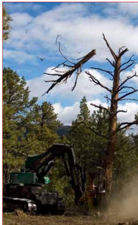
Fragile snag would prove fatal to a manual faller; but, FOPS on this feller buncher protected the operator from injury.
