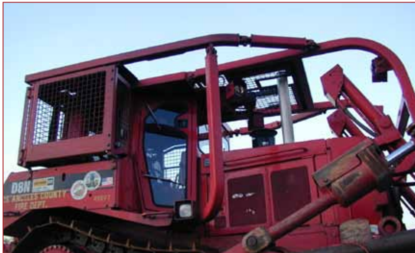
Enclosed cab FOPS/ROPS, sweeps and screens
