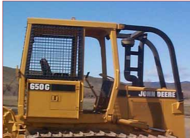
FOPS / ROPS, sweeps and partial screens
