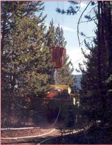
Aerial bucket remote water delivery
