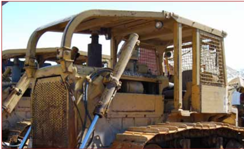
Extended FOPS/ROPS, sweeps and partial screens
