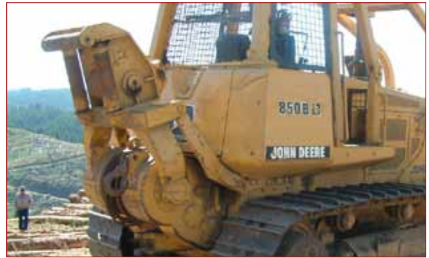
Cable Winch & Arch
