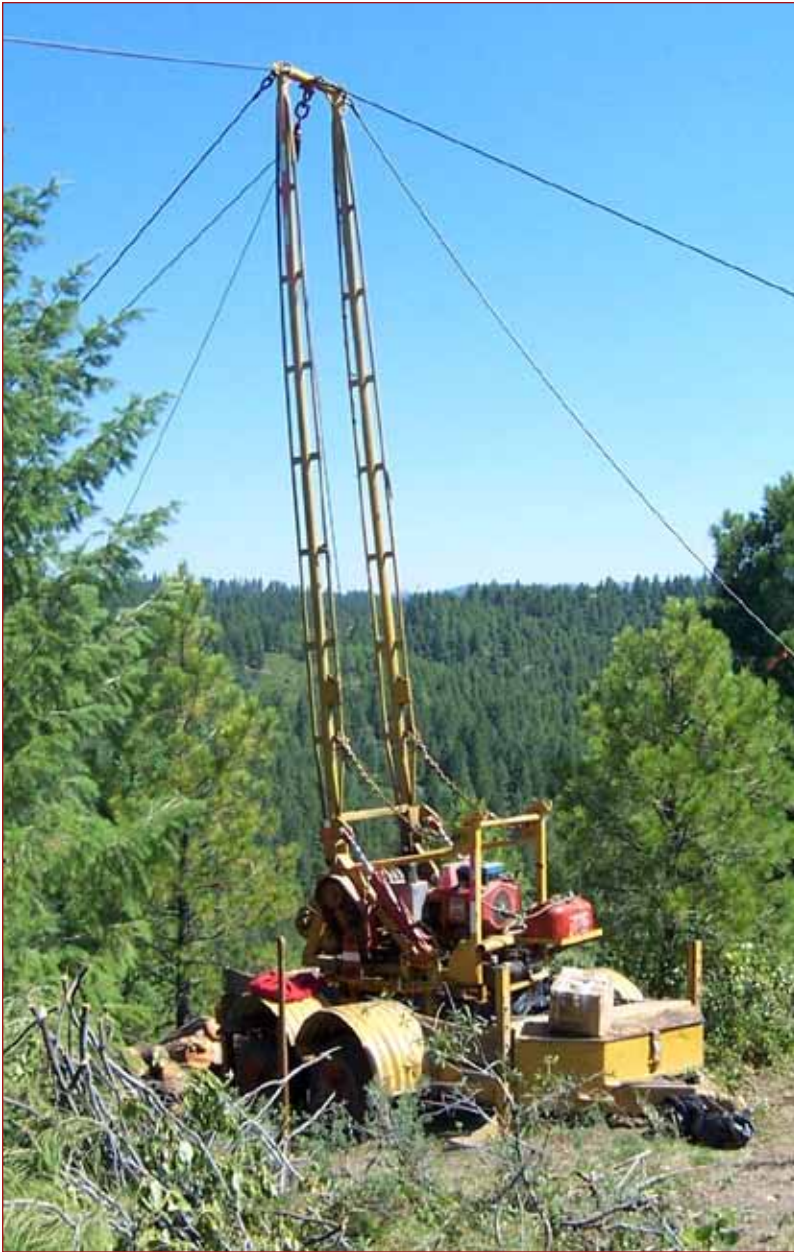
Mobile yarder for fuels reduction on steep slopes around Idaho City, ID, on the Boise National Forest
