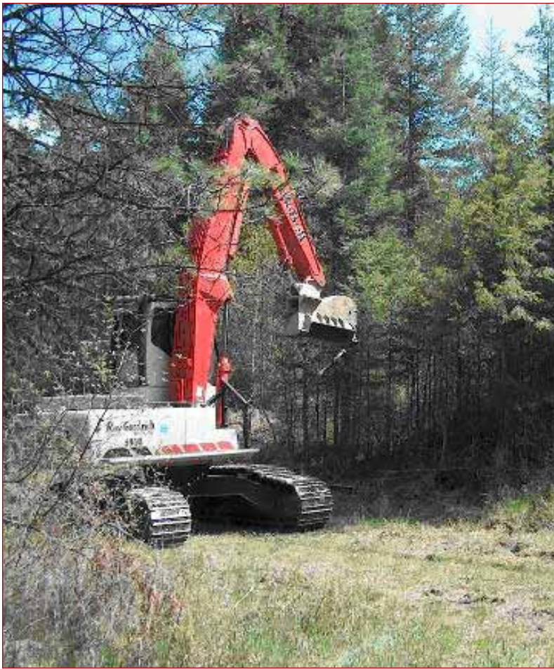
Ray Goodrich (Lenore, ID) contracted with the Nez Perce Indian Reservation to use his Linkbelt loader with a boom-mounted mulching head to reduce ladder fuels.
