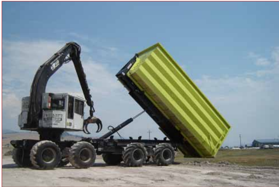
Roll-off bins for hauling slash and chips. CET Technologies Inc, Florence, MT
