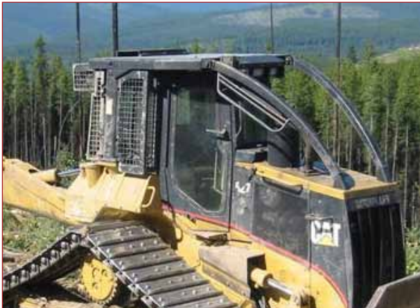
Enclosed cab FOPS/ROPS, sweeps, screens
