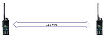
This illustration shows two units communicating with each other on a simplex channel. Both radios send and receive on the same frequency.
