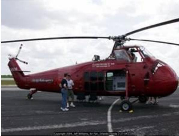
The Sikorsky S58 (H34) Choctaw was the only one used by DNR in 1971 and offered extended capability for providing larger crews and greater water capacity. This helicopter carried a 450 gallon bucket and had a 1500 horsepower engine.
