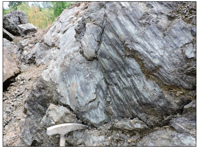
Figure 13. Slickenlines on a steeply-dipping fault exposed in the rock quarry directly north of the Carpenter Creek fault (CCF) at significant site 9M where cataclastically deformed Western mélange belt greenstone (unit tz) is exceptionally well exposed. The east-northeast strike of the fault and steep plunge of the slickenlines illustrated here are generally consistent with the CCF as a high-angle, oblique-slip fault zone with both reverse and normal movement. This brittle deformation has tectonically intercalated metavolcanic and metasedimentary rocks within the WMB. In the northern part of this large quarry, unit tz grades into less disrupted WMB away from the CCF.
