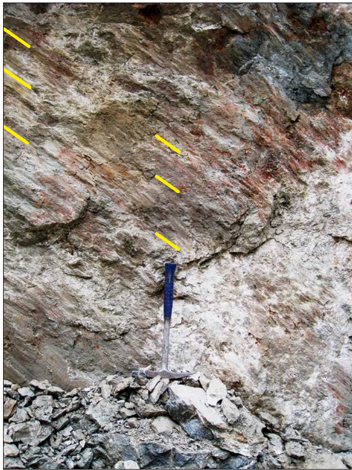
Figure 5. Slickensided face of metagabbro (unit KJigb w ) at significant site 2A, located in a rock quarry directly south of Three Lakes Hill. The deeply excavated and active rock pit exposes a fault zone (unit tz) that is subsidiary to the Three Lakes Hill fault. The faults and fractures form tectonic zones that thicken north of the pit. These faults strike east-west, are sub-vertical to vertical, and locally have slickenlines that plunge moderately to steeply southeast (slickenline rake highlighted in yellow). The slickenlines are consistent with vertical components of slip inferred on the nearby Three Lakes Hill fault.
