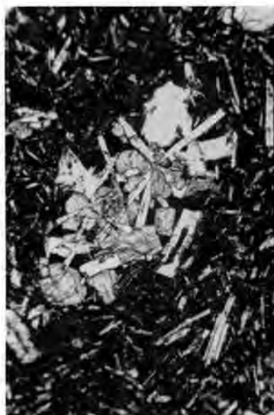
FIGURE 10. Glassy Metchosin basalt, showing cumuloaphyric texture (photomicrograph). \times 41 . Plain light.
