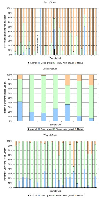
Figure 12. MQ1.3 Percent of Delivering Road Network by Surfacing. This information is also included in numerical format in Table 7.
