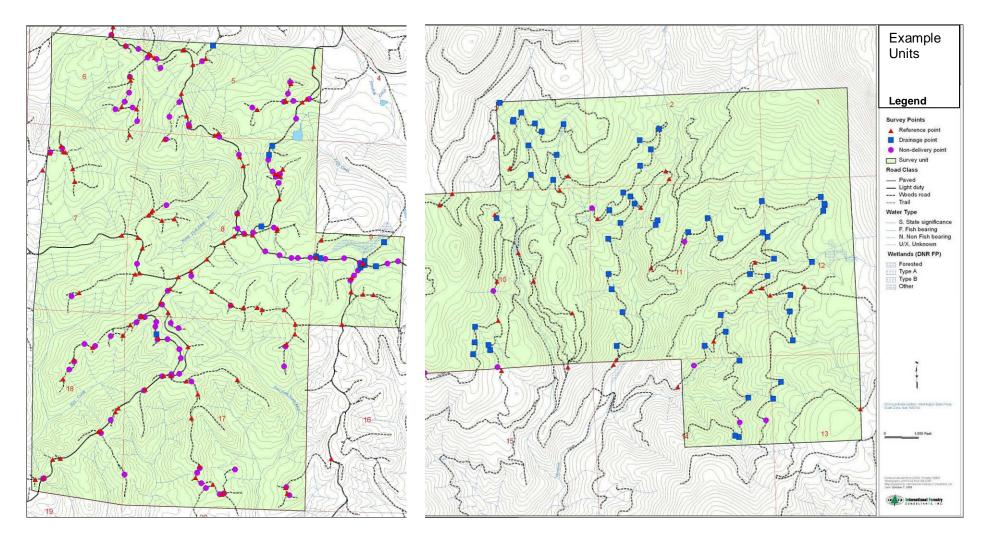
Figure 30. Sample Unit Maps Showing Difference in Delivery Between Units with Ridgetop Roads (left) and Midslope/Valley Bottom Roads (right)
