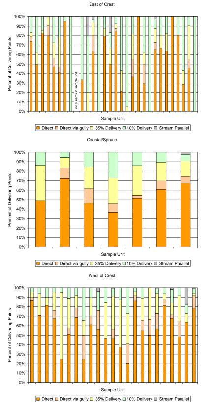
Figure 15. MQ1.6 Percent of Drainage Points by Connectivity Class. This information is also included in numerical format in Table 7.
