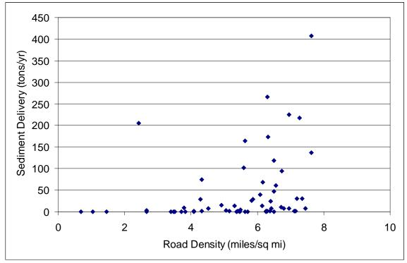
Figure 7. Estimated Sediment Delivered to Streams in Sample Unit vs. Road Density. Includes all sample units across state
