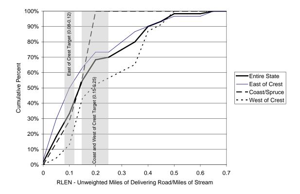
Figure 22. MQ3.1 Cumulative Percent of Sample Units, Miles of Delivering Road per Mile of Stream (RLEN).
