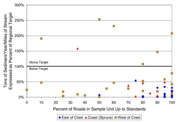
Figure 29. Tons of Delivered Sediment/Miles of Stream (MQ3.2) Expressed as Percent of Regional Target vs. Percent of Road Miles in Sample Unit Reported to be up to Standards.
