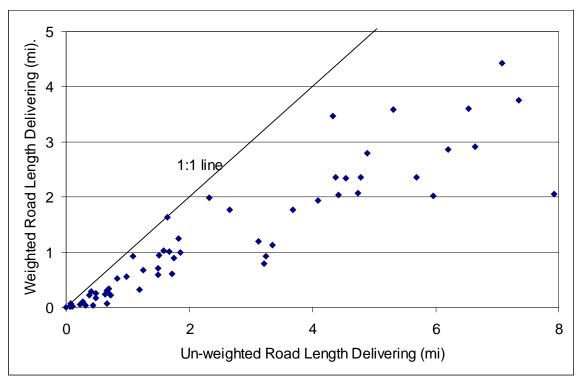
Figure 8. Un-weighted vs. Weighted Road Length Delivering for the Sample Units. Includes all sample units across state
