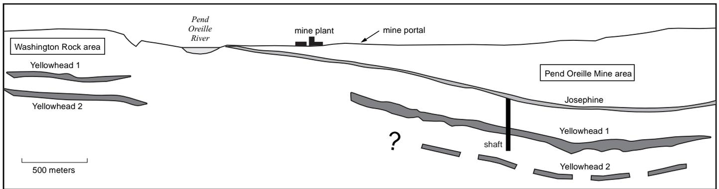
**Figure 4.** Washington Rock area to Pend Oreille mine area long section, looking northwest. Location of mineralized zones relative to the mine plant are depicted. Decline that descends from the mine portal to the Yellowhead 1 ore zone is not depicted on this section. Location of section is shown on Figure 3. (Modified from Teck Cominco website.)
