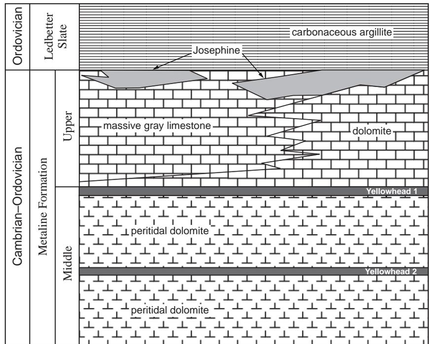
**Figure 2.** Schematic representation of stratigraphy at the Pend Oreille mine in the middle and upper Metaline Formation and overlying Ledbetter Slate. Horizons where mineralization occurs are shown relative to stratigraphic position. (Modified from Teck Cominco website.)
