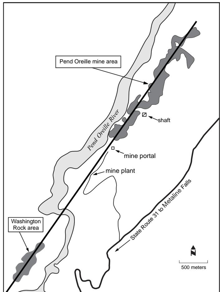
**Figure 3.** Projection of Yellowhead-type mineralization to the surface in the Washington Rock and Pend Oreille mine areas relative to the Pend Oreille River. Thick northeast-trending line is location of cross section on Figure 4. (Modified from Teck Cominco website.)
