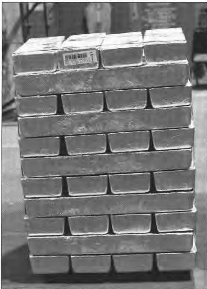
Figure 5. Magnesium metal is cast into ingots or bars for shipment. Northwest Alloys produces 35-, 50- (shown above), 250-, and 500-lb ingots. Most of the magnesium produced is shipped to aluminum plants for alloying with aluminum to make beverage cans.
