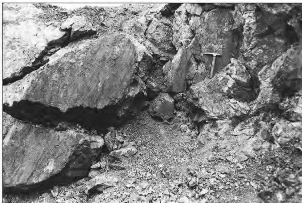
Figure 5. Slickensides in brecciated andesite in the upper level of the road-fill quarry.
