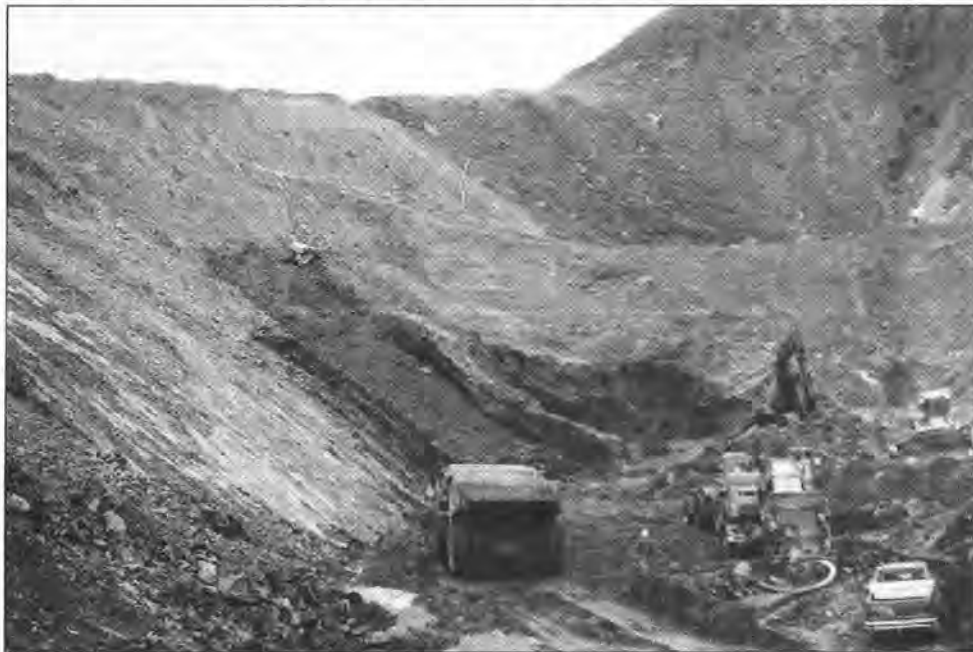
Figure 2. John Henry No. 1 coal mine, Pit No. 1, in January 1996. This view to the northeast shows mining on the southeast limb of the anticlinal structure. Light-colored ('bare rock') material to the left of the large truck forms the floor of the Franklin No. 7 coalbed. The Franklin Nos. 7, 8, and 9 coalbeds merge in this part of the mine; very little sedimentary rock separates the coals. The Franklin No. 10 coalbed is exposed in the highwall to the right out of view.
