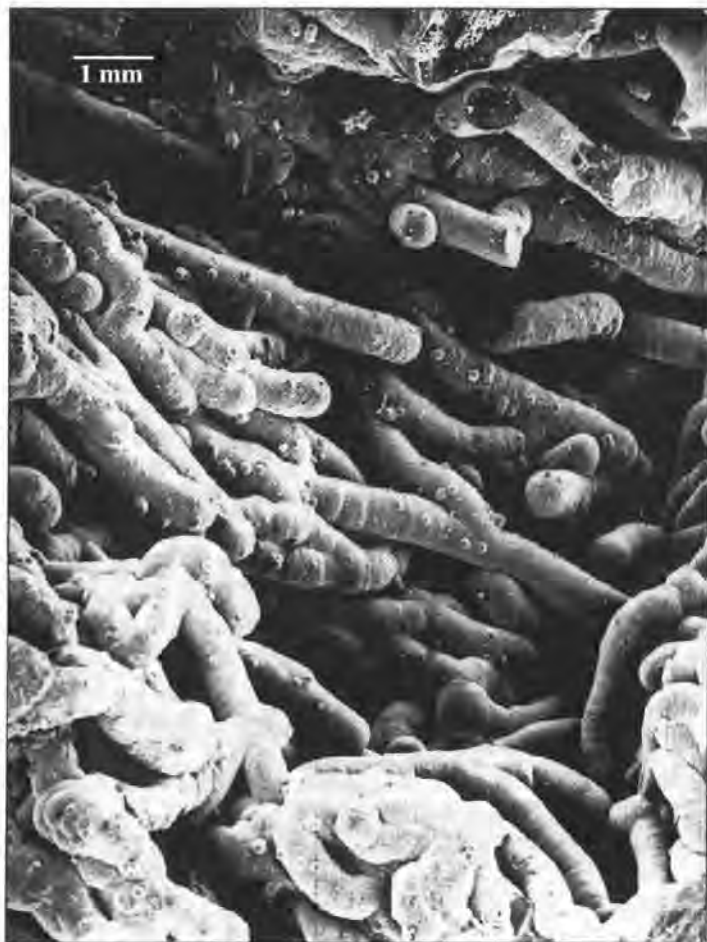
Figure 12. Scanning electron microscope photo of cristobalite encrusting chalcedony from brecciated andesite zone.
