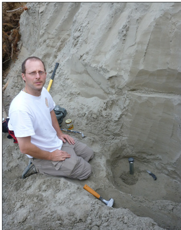
Figure D2. Rhythmically bedded, very fine sand of unit Qgos, with slump structures in the main pit wall of Asbury's Topsoil sand pit (date site GD15, sec. 13, T25N R1W). A sand sample for luminescence analysis by IRSL and OSL (Tables B2 and B3) was collected in a subpit of the main pit floor ( top left ). The pit wall exposes approximately 20 1-ft-thick rhythmmites (varves?). We interpret the bench above the main pit wall as an early shoreline of Lake Russell at elevation 420 to 400 ft. The level of the main pit floor is lateral to a later channel carved into the bench at elevation 380 to 360 ft. The sample was collected at the bottom of the subpit about 10 ft below the main pit floor and thus below approximately 30 rhythmmites at an elevation of about 340 ft.
