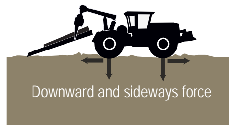
Figure 3-17. Soil Displacement; Skidder Shown
