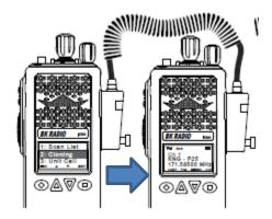
Connect the KAA0701 (or KAA0700) Cloning Cable to the side connector of the Source and Target radios and power up both radios. It doesn't matter which end is which. Use the thumb screws to secure the connectors. Avoid pulling or twisting the cable at the connectors; it will help them last.
