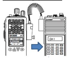
Caution > Pre April 2001 version GPH radios are not compatible as they have a different computer inside. They cannot be cloned from the P150S but can be cloned from other GPH and DPH radios.
