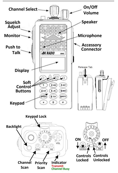
The Relm/BK KNG-P150s is a direct descendant of the GPH that is familiar to most wildland firefighters. Improvements include: increased channel capacity (32 zones of 16 channels each, up from 15 zones), decreased size and weight, greater resistance to water and dust damage and increased transmit power.
