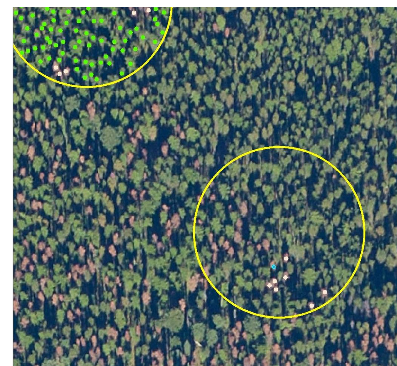
Figure 2. Screen shot showing process of digitizing live (green) and recently dead (red) trees on an orthophoto.
