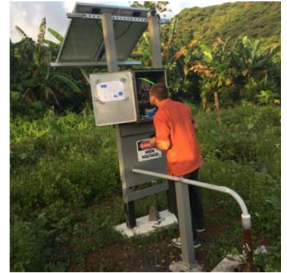
Typical American Samoa telemetered microseismic recording station checked by geoscience technician Matthew Erickson.
