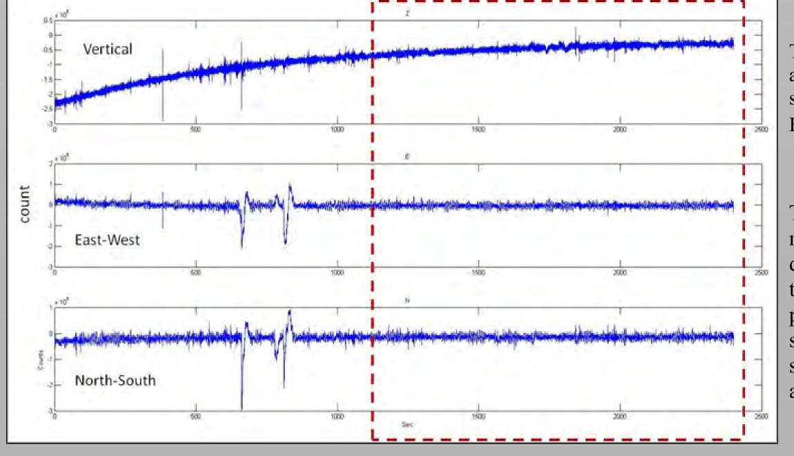
Three-component (E-W, N-S and Vertical) ambient noise recording. Dashed red box shows examples of signals used for the HVSR analysis.
