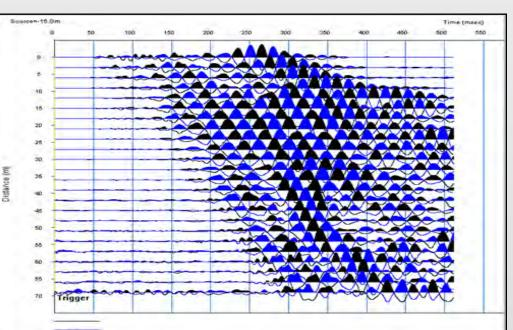
A shot gather with 180°-polarized shearwave onsets, generated by striking both ends of the wood beam coupled to the ground by parking the front two wheels of the field vehicle on the beam. First onset of the doublets show the arrival times picked for refraction analysis (Cakir and Walsh, 2010).
