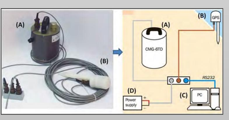
Components of the data acquisition system: (A) Guralp CMG-6TD seismometer, (B) GPS unit, (C) data recording and storage (SCREAM; data acquisition system software running on a Laptop computer), (D) battery. [http://www.guralp.com/products/6TD/]
