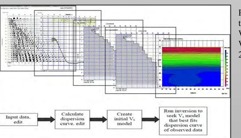
Processing steps for the Multichannel Analysis of Surface Waves (MASW) (Cakir and Walsh, 2010; Geometrics,
