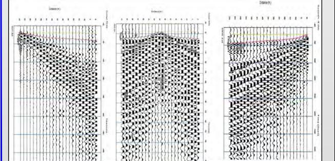
Examples of forward, center and reverse shot gathers. Red lines shows the p-wave first break picks used for the p-wave refraction analysis to estimate subsurface (shallow) Vp profiles by using two-layer or three-layer time term inversion analysis to generate initial Vp model that can be used in tomography process.
