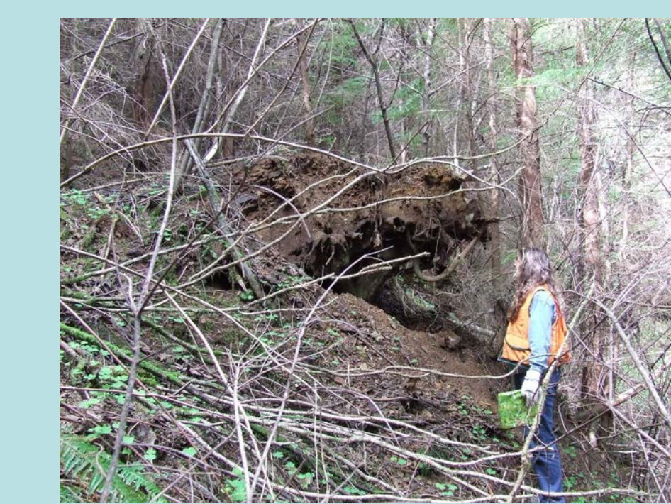
Photo above and below are 50' apart along a slope of an earthflow. Loading due to road above and additional water concentration may have activated this landslide (Chehalis Sloughs WAU).
