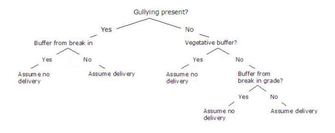
Figure B-2: Surface Erosion Delivery to Streams
