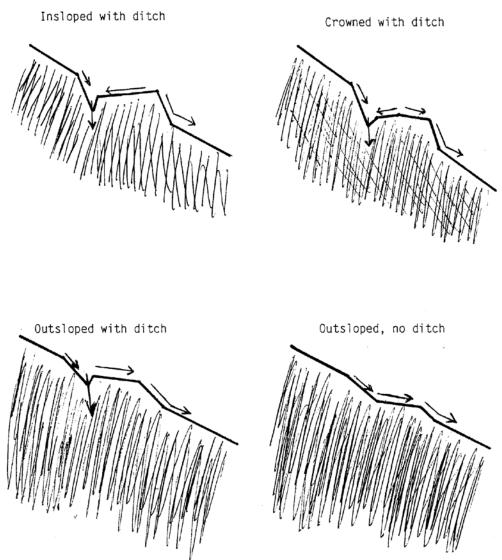
Figure B-3: Road Prism Cross-Sectional Design
