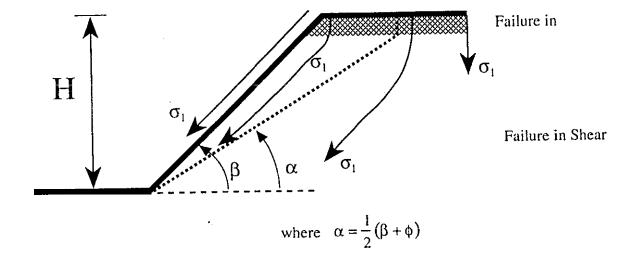
Figure 2-4. Graphical representation of input parameters in plane failure stability model adapted from Hock and Bray (1977). Because the geometry and thus the weight of the potential failure block depends on the vertical tension crack position, two versions are presented: A) headscarp in upper slope surface characteristic of failures in glacial sediments, and B) headscarp in slope face characteristic of bedrock failures in the Chuckanut Formation. Variables are explained in text and Appendix C.
