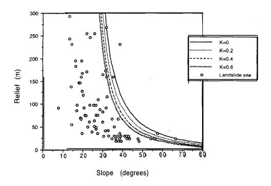
Figure 5-5. Location of LTD under range of horizontal seismic accelerations from Og to 0.6g for lithologies of the Santa Cruz Mountains assuming coseismically formed failure planes. The vast majority of the landscape is predicted to be unstable with horizontal accelerations of 0.2g or greater.
