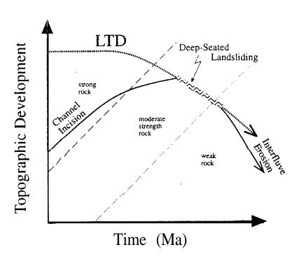
Figure 6-5. a. Limits to topographic development (LTD) (dotted line) for two different weathering rates. Low weathering rates allow high degrees of topographic development (LTD1) over long time spans while high weathering rates produce weak rock and thus less relief and gentler hillslope gradients (LTD2).
