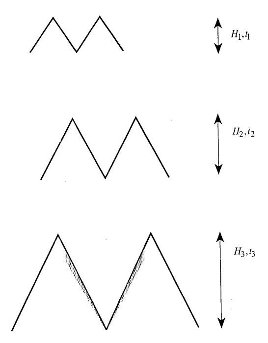
Figure 2-6. Limit to topographic development (LTD) defined by features of observed topography (hillslope gradient and relief). The LTD relief asymptote is determined by the friction angle while the slope asymptote is controlled by cohesion.
