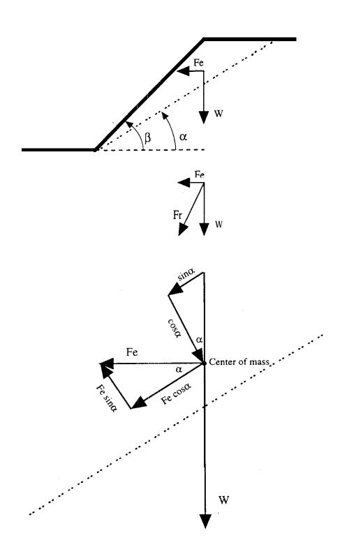
Figure 5-2. Force due to earthquake, Fe, expressed as an equivalent static force with magnitude KW, where K is **the** seismic coefficient and W is the weight of the failure block. A moderately destabilizing condition is depicted with Fe is oriented vertically downward. Fr denotes the resultant force. Dashed line represents potential failure plane.
