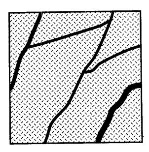
Figure 6-2. Hypothetical rock mass strength distribution. Small samples are dominated by average strength values while large samples also possess the tail ends of the strength distribution.
