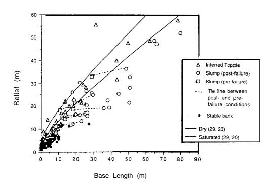
Figure 3-7. Schematic interpretation of Figure 3-6a showing spatial distribution of hillslope processes in the context of topographic development. Sites located above the saturated threshold may be highly susceptible to hydrologic changes within the watershed.
