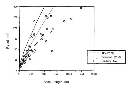
Figure 3- 18. Graphical representation of Coulomb equation for **Quaternary glacio- fluvial** deposits, anti-dip and dip slopes of the Chuckanut Formation, and sedimentary units of the Santa Cmz Mountains.
