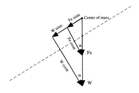
Figure 5-3. Force due to earthquake, Fe, expressed as an equivalent static force with magnitude KW, where K is the seismic coefficient and W is the weight of the failure block. A stabilizing condition is depicted with Fe oriented vertically upward. Fr denotes the resultant force. Dashed line **represents** potential failure plane.
