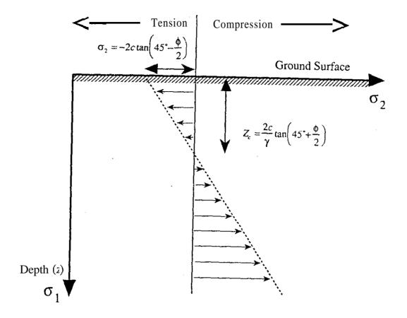
Figure 2-3. Wedge-shaped landslide block defined by planar failure surface (dashed line) intersecting zone of tension determined by Rankine theory. From the surface to shallow depths the gravity-induced principal stresses  $\sigma_l$  is oriented approximately parallel to hillslope of unvarying inclination,  $\beta$ , and the failure surface is inclined at  $\alpha = \frac{1}{2}(\beta + \phi)$  to the horizontal Failure represents conditions satisfying the Culmann model.
