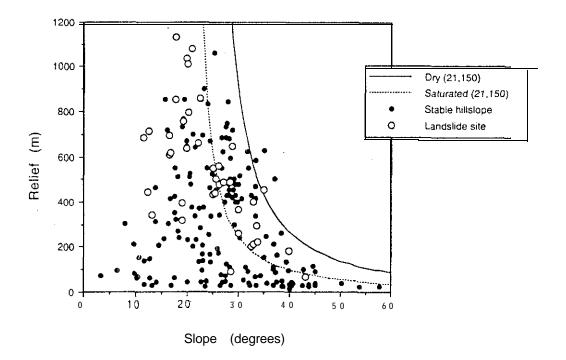
Figure 3-12. a. Anti-dip slope transects for the Chuckanut Formation plotted with respect to gradient and relief. Values reported to right of thresholds refer to friction angle,  $\phi = 21^{\circ}$  and cohesion,  $c = 150 \, \text{kPa}$ .
