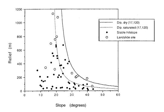
Figure 3-13. a. Anti-dip slope transects for the Chuckanut Formation plotted with respect to base length and relief. Values reported to right of thresholds refer to friction angle,  $\phi = 21^{\circ}$  and cohesion,  $c = 150 \, \text{kPa}$ .
