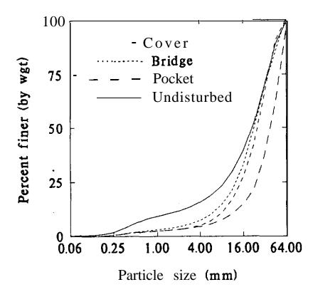
Figure I-A- $\sim$ . Cumulative distribution (combined sample dry weights) for 29 egg pockets in the spring.
