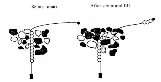
Scour during peak flows occurred on all cross-sections in all habitat types. The average depth of scour for all cross-section monitors was 0. **11 m** (range 0.0-0.6 m). The average depth of scour in Reach B (0. **14** m) was nearly double that of Reach A (0.8 m). Scour at 19.7% of the monitors reached a depth of 0.2 m, the median depth of chum **salmon** egg pockets (Chapter I-A). Scour at 27.9% of the monitors in Reach B reached 0.2 m, compared to only 9.1% in Reach A.
