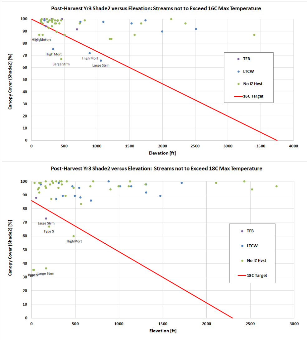
Figure 36. Canopy Cover for each site plotted versus elevation and displaying the western Washington temperature nomograph targets for streams that are subject to the 16C (top graph) and 18C (bottom graph) temperature standards. (WA FPB 2000, Section 1, Fig 1.2)
