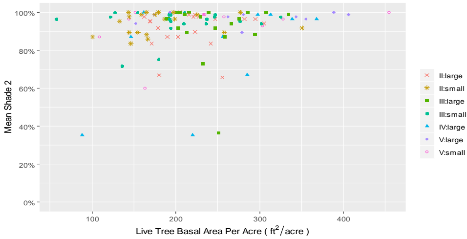
Figure 25: Shade 2 densiometer canopy closure as a function of live tree basal area, site class, and stream width category.
