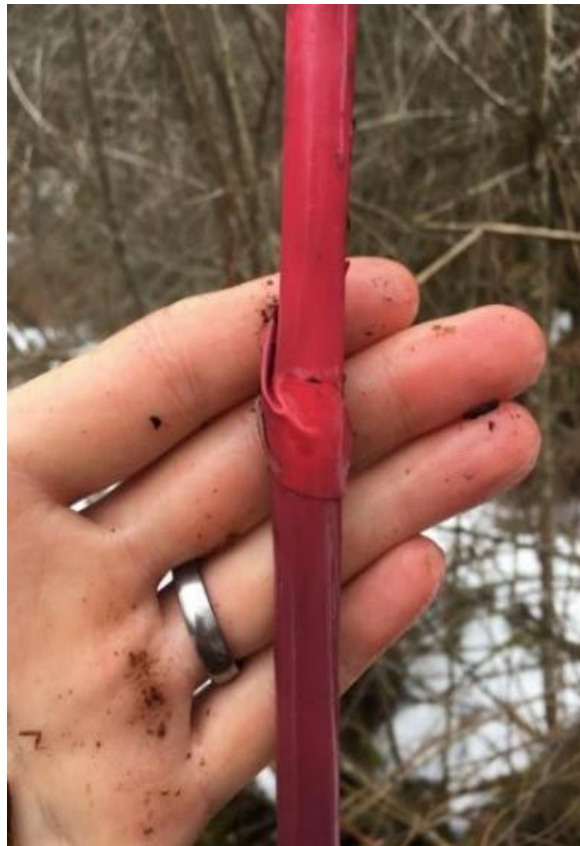
Figure 57. Gray discoloration on red PVC electrical tape (bottom) caused by reducing conditions.
