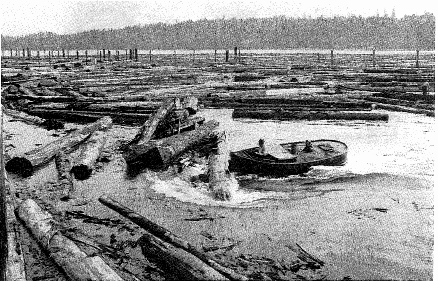
PHOTOGRAPH 7. Early boom boat breaking a "jackpot." Note log scaler on the right. COURTESY WEYERHAEUSER ARCHIVES
