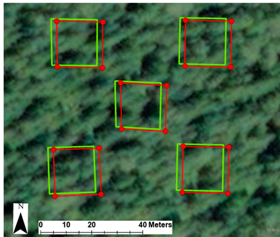
Figure 5. Example unit (containing 5 tree plots) showing the difference between the tree plot locations in the original, framework survey data and the tree plot locations using our LiDAR-based methodology. Light green rectangles represent tree plot locations from the framework survey; red rectangles represent tree plot locations after matching stem maps to LiDAR CHMs. Each unit was shifted based on the average differences between original tree plot locations and LiDAR-based locations.
