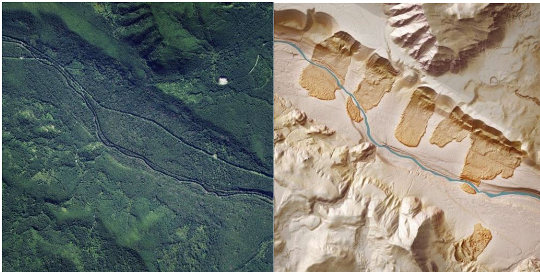
Figure 2: Comparison of imagery and lidar data over Cedar River, King County. Lidar data reveals several landslide features beneath the vegetation
