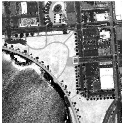
Figure 14: Example of a lidar intensity image, which represents the strength of the returned measurement to the lidar system.
